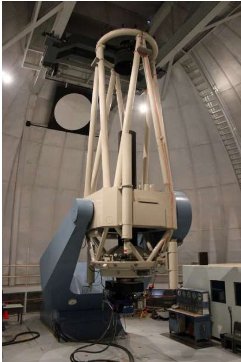
The 1.55-meter (61-inch) Kaj Strand Astrometric Telescope at the U.S. Naval Observatory Flagstaff Station (NOFS). Completed in 1964, it remains the largest instrument of its kind in the world.
